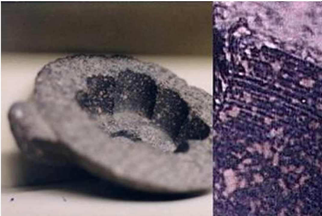
Figure 99. Tube-drilled piece of granite (Mohs scale hardness 6–7) displaying spiral grooves characteristic of tube-drilling – how?
